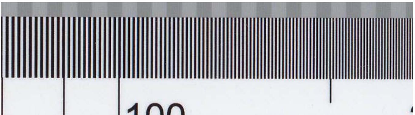
400 dpi scan of 50x chart, printed on the Epson 1270 at 1440 dpi, shown between 80 and 200 lp/mm.
