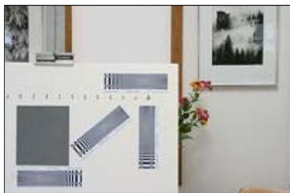
Draw a *scale* on the target to represent the distance from the center of the sensor in 1 mm increments. For the target in the illustration, which uses 5 cm charts intended for 50x magnification, the 1 mm marks were placed every 5 cm. The center of the target in the photograph (easy to locate in the viewfinder) is placed just below the number 0 on the scale, near the upper right of the target.
